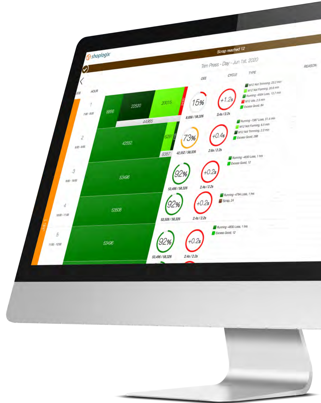
The Machine Level Whiteboard screen displays production count charts, goal and cycle gauges, downtime reasons, and comments at the Machine Level.
