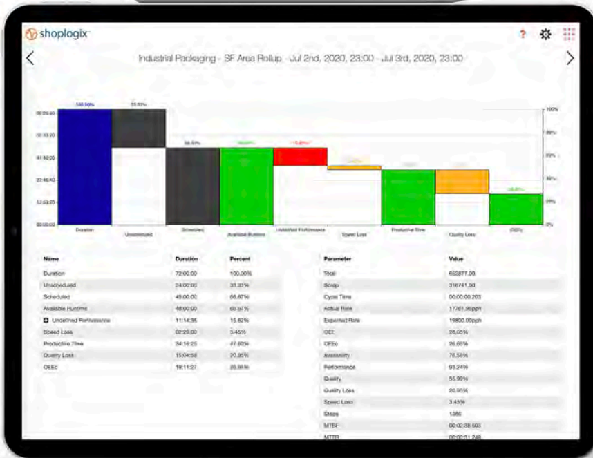
The OEE Waterfall displays loss categories and breaks down all categories of production that make up a specific machine, area, or line. The display breaks down into availability, performance, and quality.
